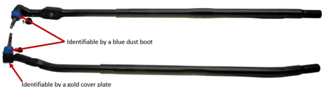
For recalled ACDelco right outer tie rod ends still in your parts inventory, please follow parts return procedures as described in ACDelco bulletin 18D-077 dated June 30, 2018. A replacement outer tie rod, part number 45A7140, will be available for ordering in November 2018.
